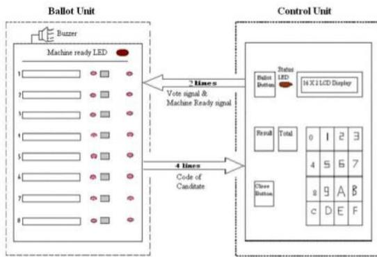
FIG 3.1 Microcontroller based EVM
