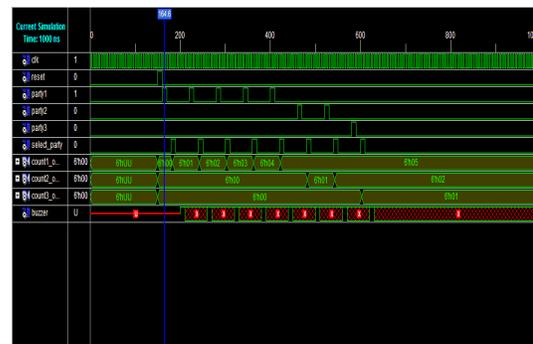
FIG XX. Simulation Result for proposed EVM
