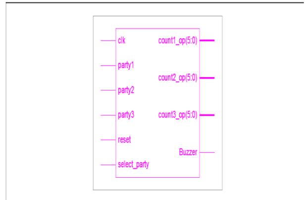
FIG Y. RTL Schematic for proposed EVM
